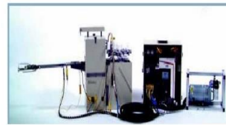
Stack gas sampler
