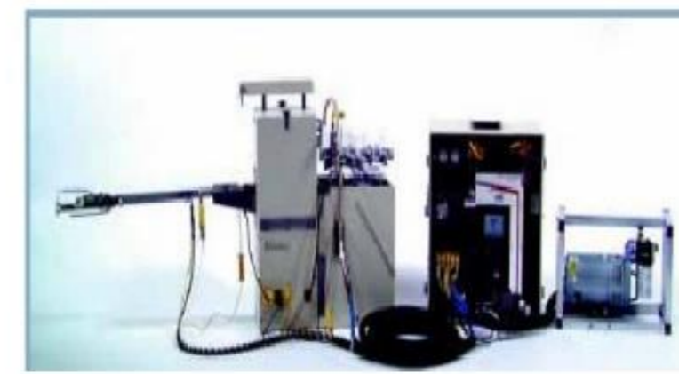
Stack gas sampler
